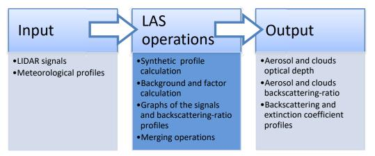
Figure 1.1: Scheme of the LAS principal characteristics
