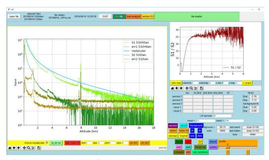
Figure 5.3: multiple signal files loaded and showed on the principal graph. The auxiliary graph shows the ratio between the two signals.
