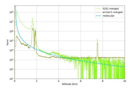
Figure 3.3: the cloud layer and the aerosol layer cannot be clearly distinguished.
