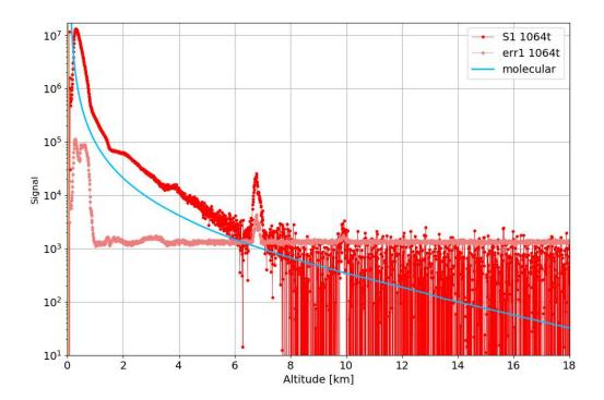
Figure 5.2: The main graph after a successful load of the signal and meteorological files. The RCS is in red, the signal uncertainty in pink and the molecular range corrected signal in light blue. Note: the colours change accordingly to the showed channel (1064 nm in this picture).
