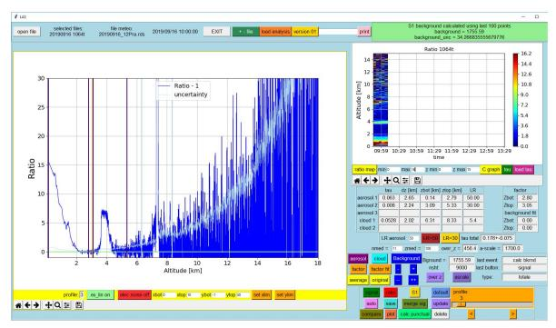
Figure 5.5: The backscattering ratio resulting from the analysis. The aerosol layer borders are marked by purple lines, the clouds borders are marked by cyan lines while orange lines mark the region in which the factor has been calculated. The cyan line represents the uncertainty. The auxiliary graph shows the backscattering ratio value as function of time and altitudes.
